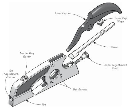
Figure 1: Shoulder plane components.
