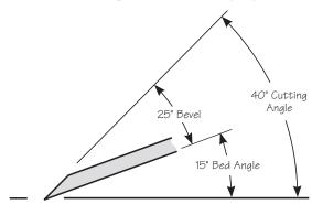
Figure 3: Blade geometry as supplied.
